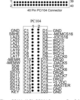
Figure PC104: 40-Pin PC/104 Connector Bus C & D
